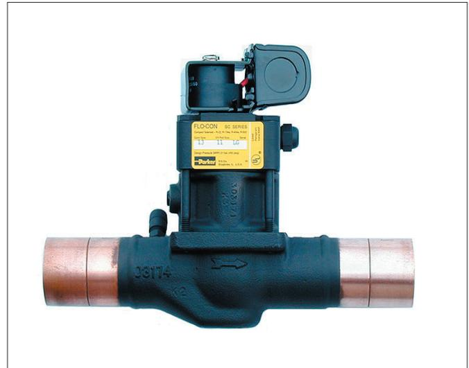
iron-bodied solenoid valve with brazed copper couplings is suitable for most common refrigerants, certain oils and other fluids approved for use in refrigeration. This valve may be opened by means of a manual opening stem in case of electrical power failure or for servicing.
